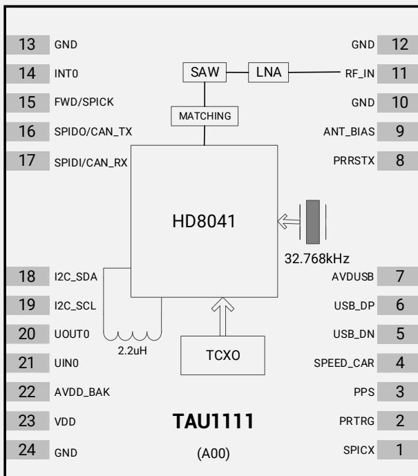
**Figure 2 Block diagram**
