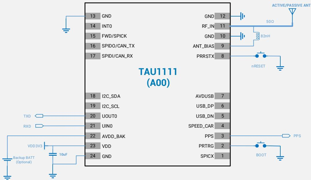
**Figure 7 Minimal application diagram**
