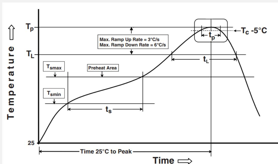
**Figure 9 Reflow soldering profile (Refer to IPC/JEDEC J-STD-020E)**
